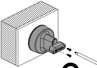
Secure the connection between the scooter's power cord and the power outlet using the provided screws and a screwdriver (C).
