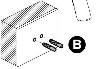
Install the mounting hardware (B) into the two holes drilled in the wall.
