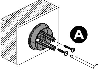
Mount the power outlet (A) onto the wall using the included screws and a screwdriver.
