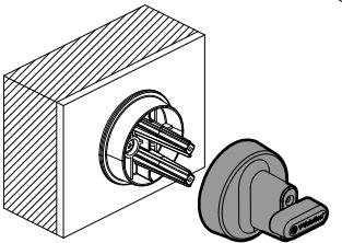
Connect the power cord from the scooter to the power outlet.
