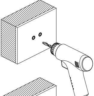
Drill two holes in the wall where the power outlet will be installed.
